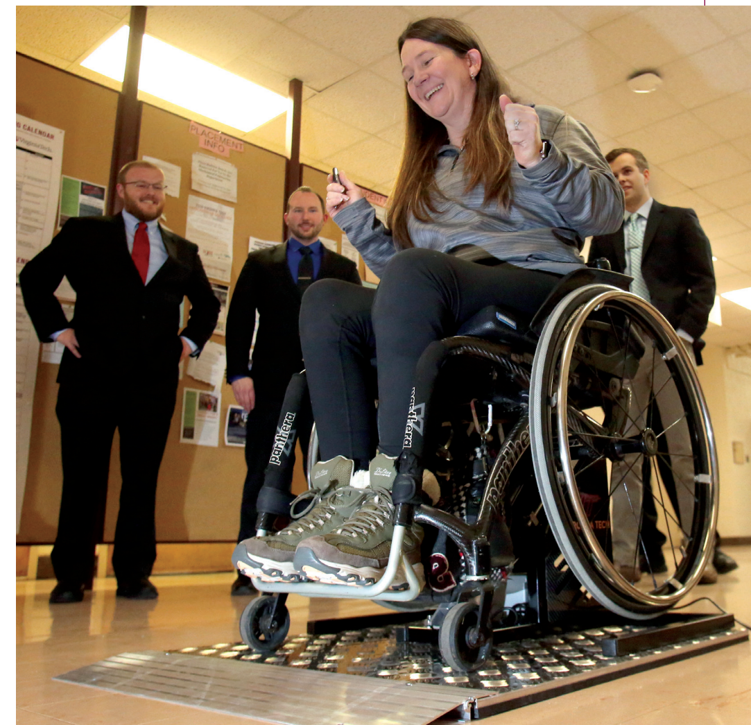
QUICK CHANGE : (top left) A team of seven engineering students, including Riley Allison '18, tests their senior design project, a tool to make changing wheelchair tires a little easier. (top right) The device, which is operated by a remote keychain fob, works like a hydraulic tire jack, pushing the chair off the ground at the axle to allow for easier wheel replacement. (above) Tammy Landeen, of Caribou, Maine, expresses joy after performing a successful wheel change independently.
